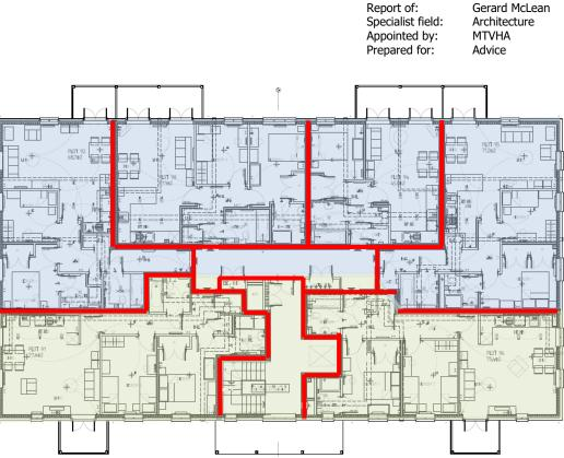
2.4 The internal walls and doors resisted the spread of fire more effectively than the external walls. While the flats to the south west of the circulation corridor were almost completely destroyed, those to the north east suffered little direct damage from the fire: they were damaged by smoke, and by firefighting water, and the structure as a whole became unstable, but the fire was held back on this line for a reasonable period of time.
